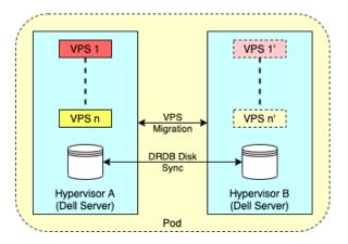
Our Pod architecture is dual machine set-up that replicates the disk used by the operating system. Should the active hypervisor machine fail, or disk fail, the VM is started up on the sibling hypervisor server. Swapping hypervisor servers is tested regularly as reboots are necessary when updating OS/kernel software. Critically, it also decreases the impact of any other customer as customers aren't sharing a single SAN.
